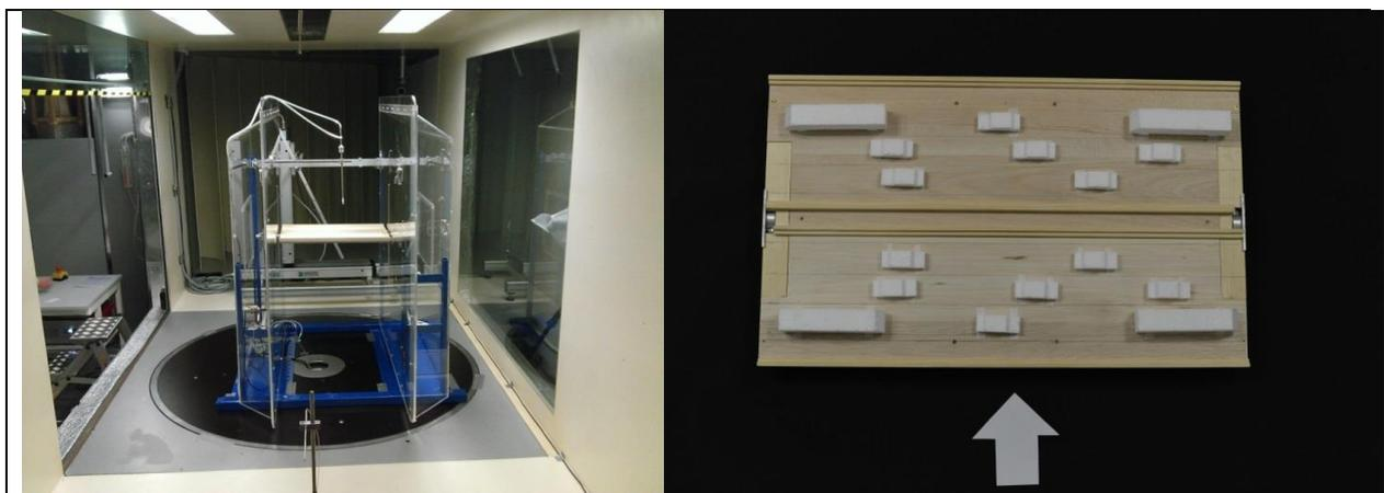
Left-Experimental set-up. Right- Model of the traffic on the bridge
