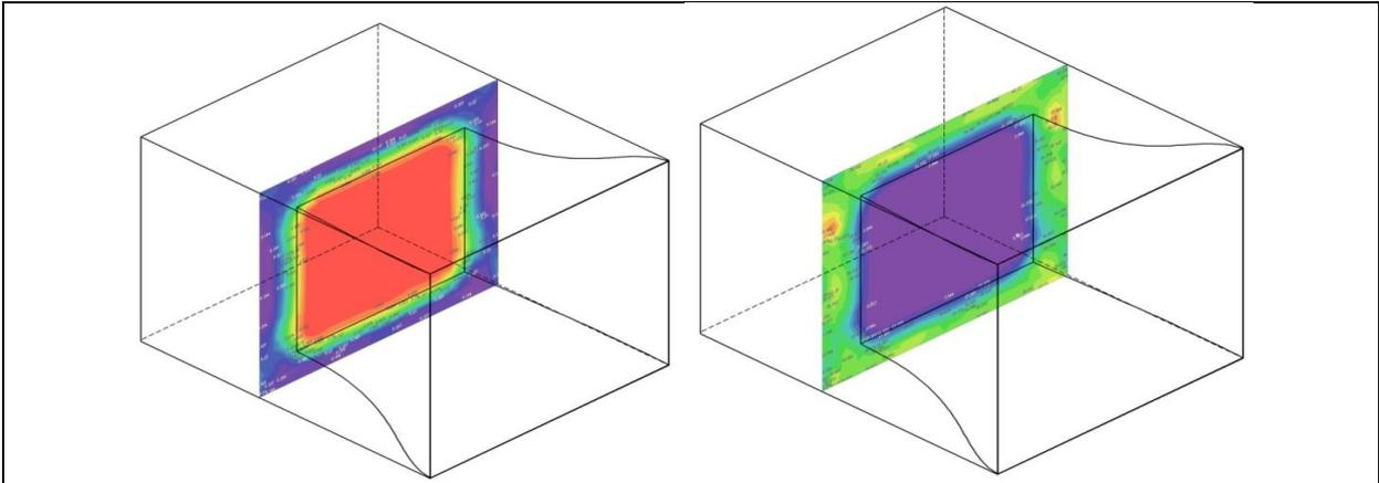
Flow characteristics of the working part: a) velocity; b) turbulence
