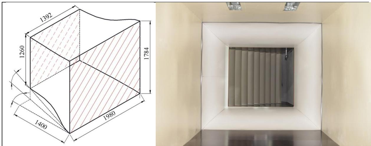
Left-Geometrical parameters of the contraction. Right- Test part of the aerodynamic section of the Climatic Wind Tunnel "Vincenc Strouhal" (downstream view)
