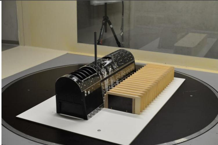
Power plant building model placed in a testing section of the wind tunnel.
