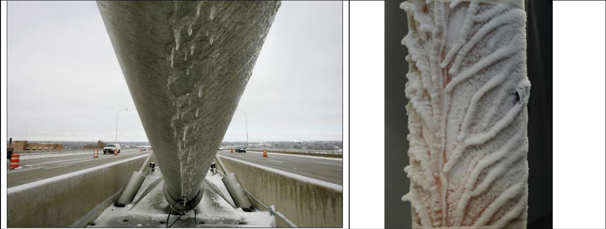
Real situation ice formation, unassisted ice accretion in the wind tunnel
