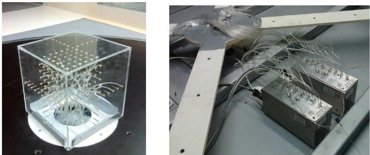
The model in the measuring section and a detail of the measuring pressure scanner below the testing section
