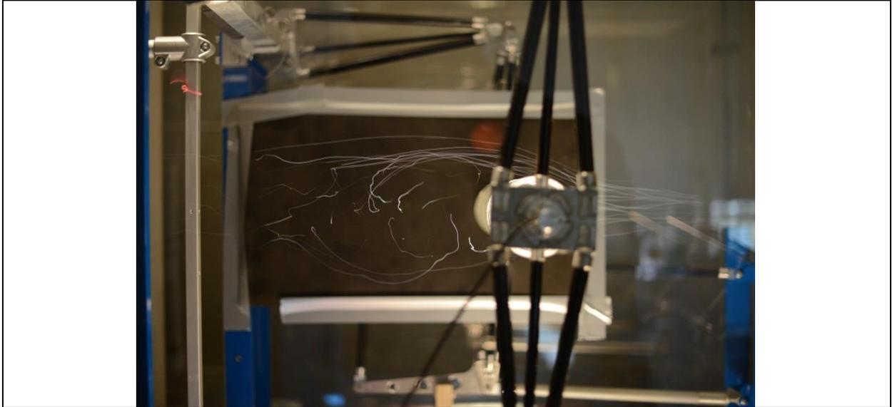
Helium bubbles tracking around a circular cylinder
