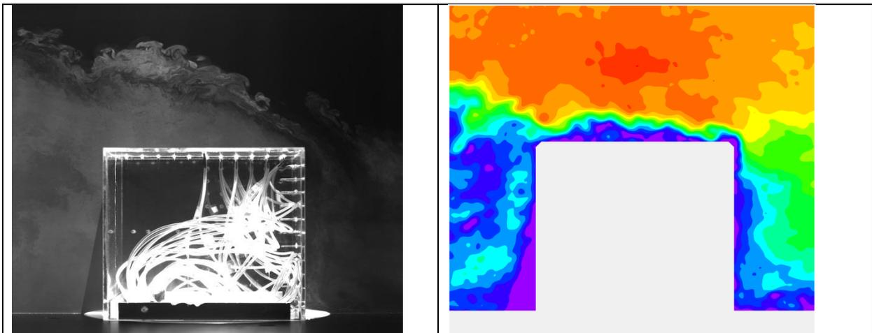
Exampe of the results of Particle Image Velocimetry technique describing the flow around a benchmark object (cube)
